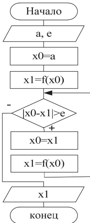
$$\text{pr\_it}(f, a, e) := \left| \begin{array}{l} x_0 \leftarrow a \\ x_1 \leftarrow f(x_0) \\ \text{while } |x_0 - x_1| > e \\ \quad \left| \begin{array}{l} x_0 \leftarrow x_1 \\ x_1 \leftarrow f(x_0) \end{array} \right. \\ x_1 \end{array} \right.$$
